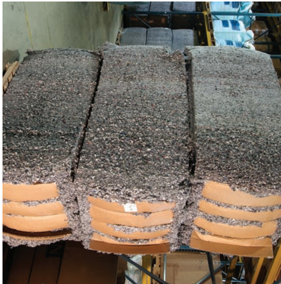
Nike Grind material is produced from old athletic shoes. They are sorted (left page) before processing. The finished product is put into bales (above).
